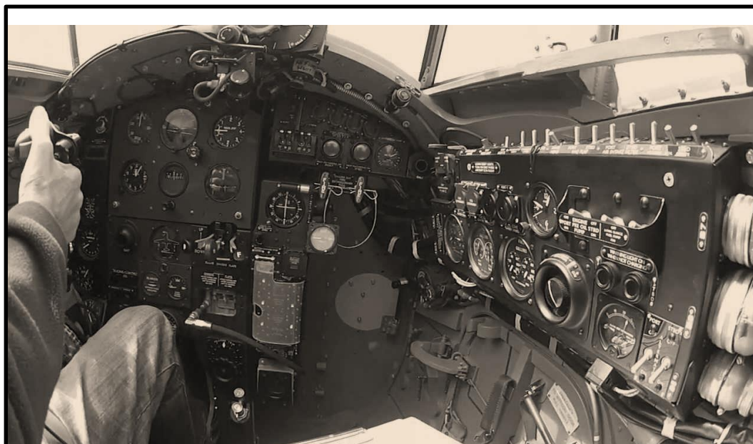
Cockpit layout of a de Havilland Mosquito, photo taken from navigators seat
