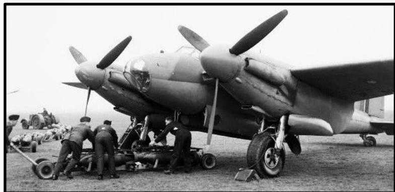
Mosquito being loaded with 500lb (220kg) bombs
